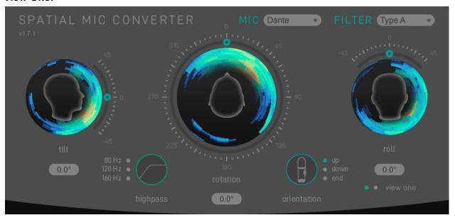
View one shows Direction Of Arrival information around the heads. This will help to understand where different sounds in the soundfield are coming from, with the brighter red color indicating the higher signal levels.
