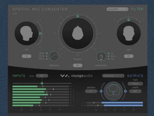
The included Spatial Mic Converter plugin transforms the raw audio signals from Spatial Mic to first or second order ambisonics. The plugin offers the capability to change the microphone's aim and decode to microphone patterns & surround formats like 7.1.2.
