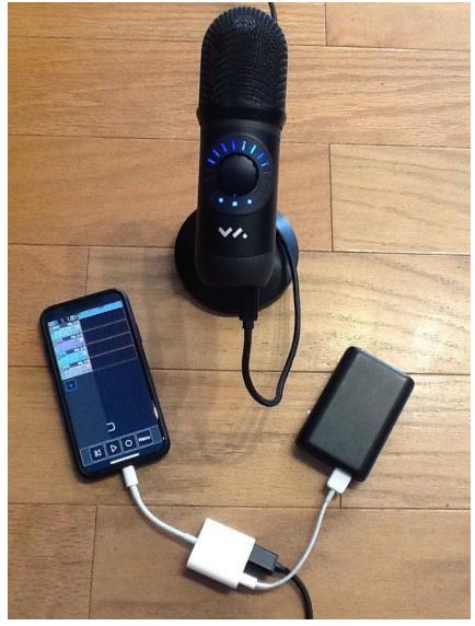
Note that the battery may also be plugged directly into Spatial Mic, however plugging the battery into the Adapter as shown will also charge the mobile device.
