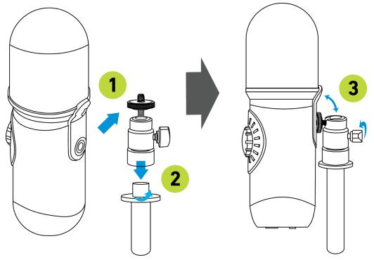
For acoustic isolation, use a Rycote InVision shockmount (sold separately). Place Spatial Mic in the shockmount so the bottom of the mic is flush with the inner shockmount ring and tighten the screws around the mic. Ensure microphone cannot slip out of shockmount and knob can be accessed.
